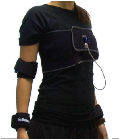
IMUs at strategic positions on body (accelerations, angular rates)
